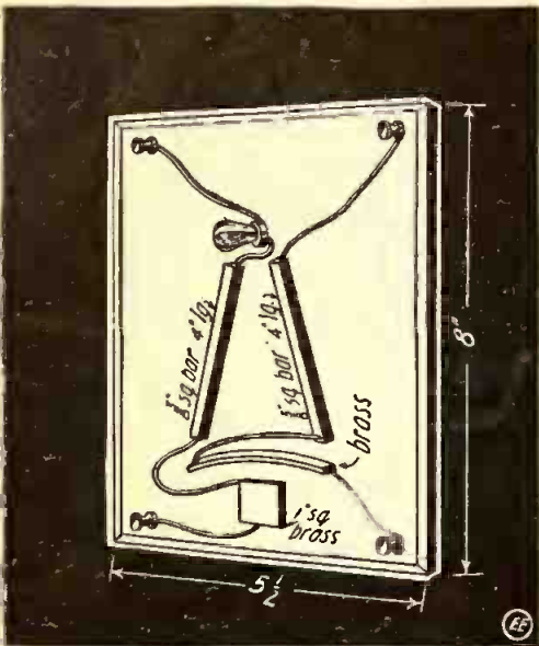
Quick Test Board for Fuses and Lamps.
