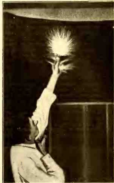
Fig. 9. Wonderful Brush Discharge Effect Produced by High Frequency Current.
